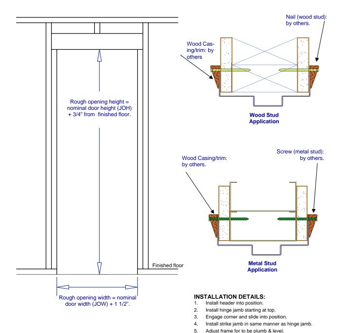
SOF provides the strength and rigidity of a commercial steel frame with an easy installation while allowing you to simply add wood trim around the perimeter for a finished decorative looked.
